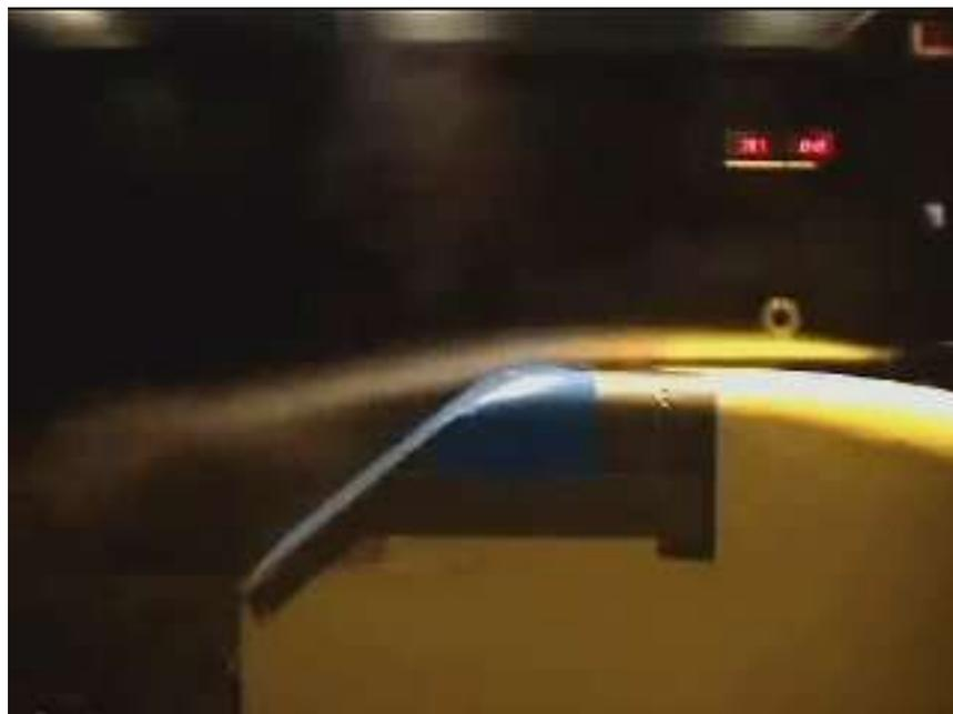
**Figure 11: The airflow clearly separates when VGs are removed from the 40° boat-tail.**
