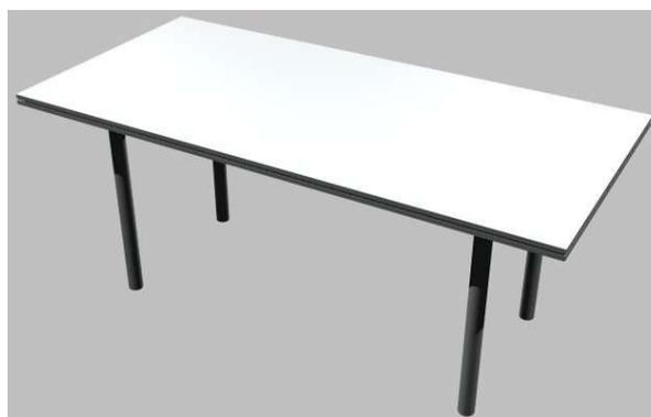
Figure 8: General description of the wind-tunnel balance used at tests in Västerås. The loading cell that measure the aerodynamic drag is mounted between the two plates at the top of the balance and the model is rigidly mounted on the top plate.
